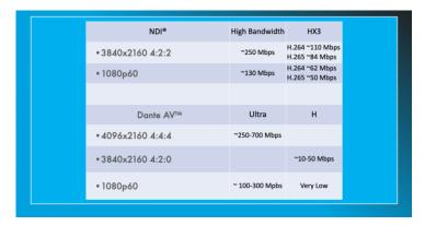
**Bandwidth is a foundational issue,** especially in the standard 1Gbps networks in which NDI and Dante AV are designed to work, and your choice of transport system must include the typical bandwidth for the video stream. The details in this table are best estimates based on my tests and sourced from NDI and Audinate.
