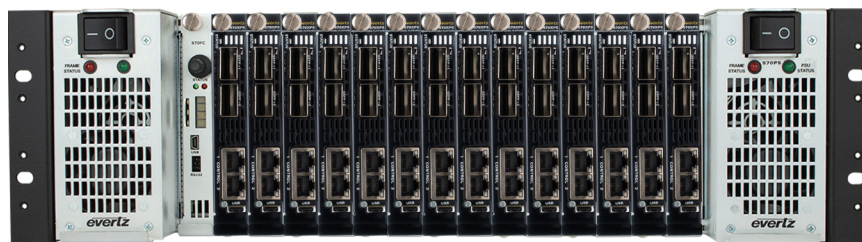
5782XPS encoder and decoder blade, shown with fully loaded 3RU chassis
