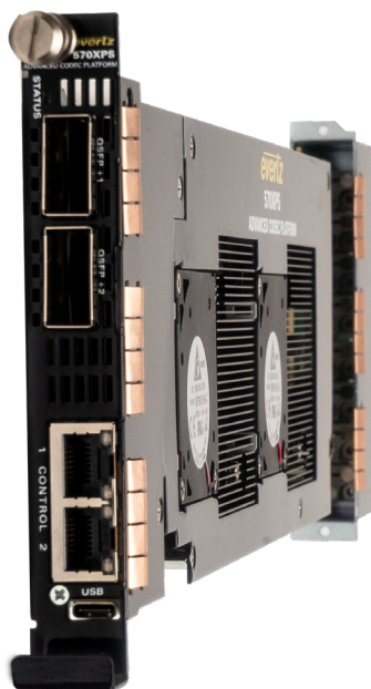
5782XPS encoder and decoder blade, shown with fully loaded 3RU chassis
