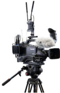
The meshLINK hardware mounted on a professional camera.
