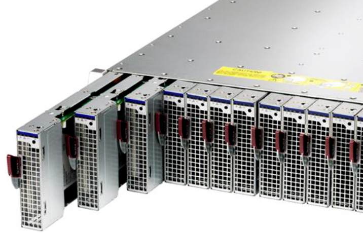
Fully modular chassis with 14 hot-swap encoding modules
